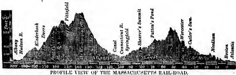
PROFILE VIEW OF THE MASSACHUSETTS RAIL-ROAD.
